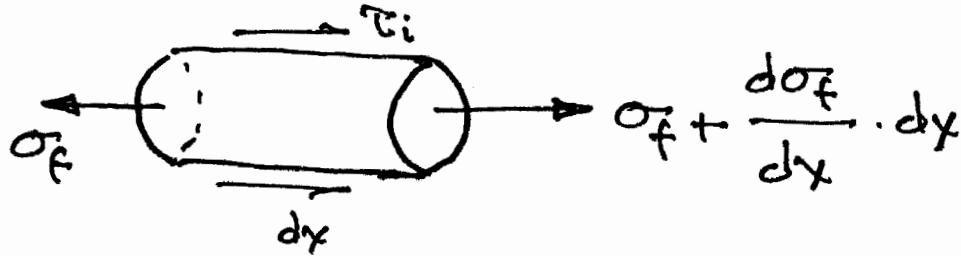
$$\left( \frac{d\sigma_f}{dx} \cdot dx \right) \frac{\pi d^2}{4} = -T_i (\pi d) dx \rightarrow \frac{d\sigma_f}{dx} = -\frac{4}{d} T_i$$
