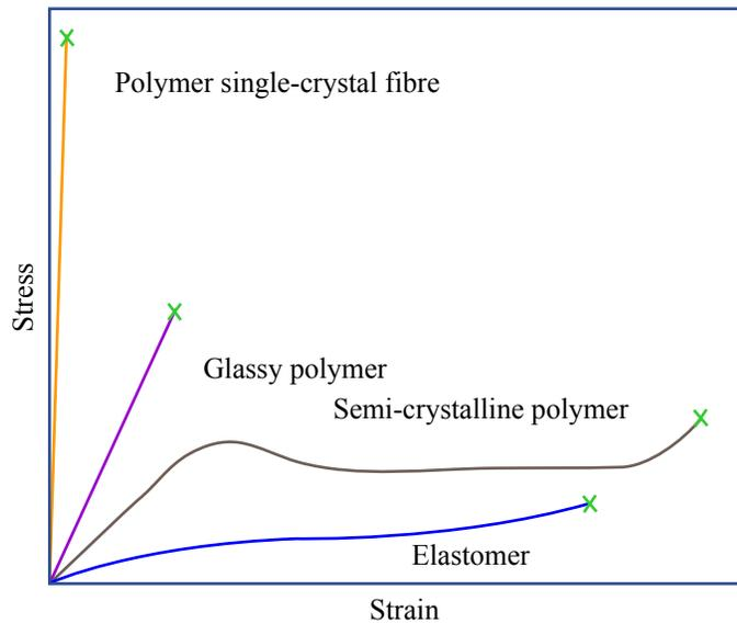
*Schematic stress-strain curves of different types of polymers, drawn approximately to scale.*
