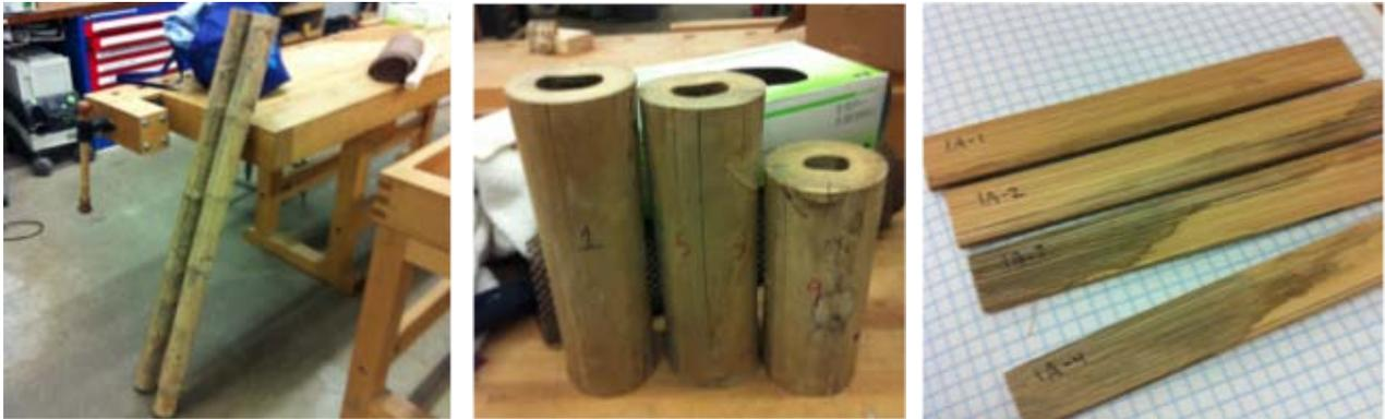
**Figure 3.1** *Left:* Tre Gai bamboo before splitting. *Middle:* Internodes 1, 5, and 9. *Right:* Finished samples for three-point bending.
