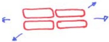
loading at  $\theta^\circ$  to struts  $E^* \propto E_s(\rho^*/\rho_s)^3$
