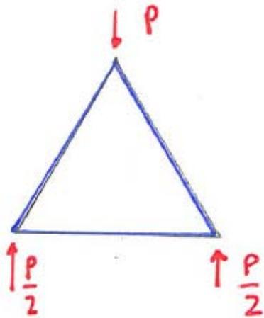
$$\sigma \propto \frac{P}{lb} \quad \epsilon \propto \frac{\delta}{l} \quad \delta \propto \frac{Pl}{AE_s} \text{---axial shortening: Hooke's law}$$
