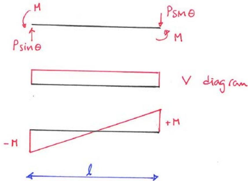
M diagram: 2 cantilevers of length  $l/2$
