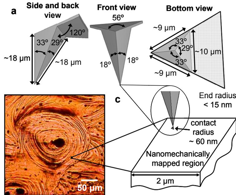
Silicon tetrahedral probe tip indenter ( $k \sim 56 \text{ N/m}$ )
