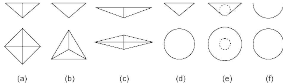
a=Vickers, b= Berkovich, c= Knoop, d = conical, e=Rockwell, f=spherical
