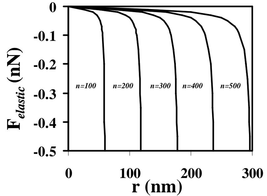
(left) Elastic force versus displacement as a function of the statistical segment length,  $a$ , for the non-Gaussian FJC model ( $L_{contour} = 200$  nm) and (right) elastic force versus displacement as a function of the number of chain segments,  $n$ , for the non-Gaussian FJC model ( $a = 0.6$  nm)
