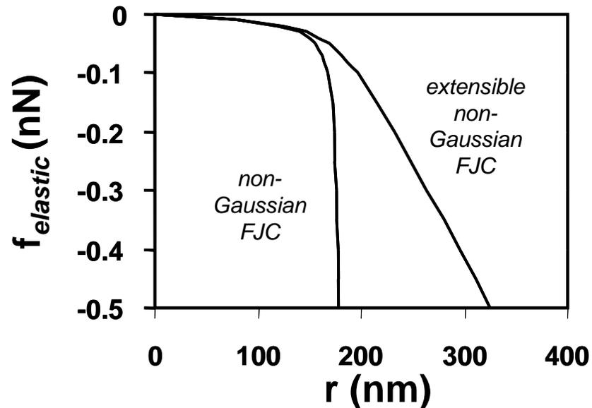
Schematic of the stretching of an extensible freely jointed chain and (b) the elastic force versus displacement for the extensible compared to non-extensible non-Gaussian FJC ( $a = 0.6$  nm,  $n = 100$ ,  $k_{segment} = 1$  N/m) - note units
