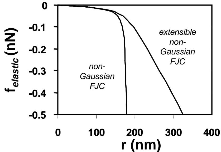
Schematic of the stretching of an extensible freely jointed chain and (b) the elastic force versus displacement for the extensible compared to non-extensible non-Gaussian FJC ( $a = 0.6$  nm,  $n = 100$ ,  $k_{segment} = 1$  N/m)
