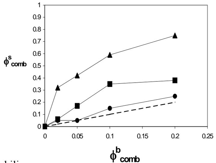
PLA scaffold with surface segregated amphiphilic comb copolymer. SEM image (left) and XPS data of comb surface vs. bulk concentration. (D.J. Irvine et al., *Biomacromol.* **2**, 545 (2001))
