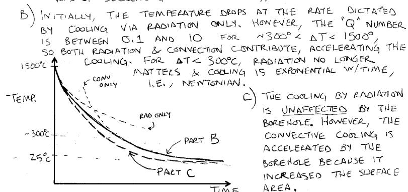
THE COOLING BY RADIATION IS UNAFFECTED BY THE BOREHOLE. HOWEVER, THE CONVECTIVE COOLING IS ACCELERATED BY THE BOREHOLE BECAUSE IT INCREASED THE SURFACE AREA.
