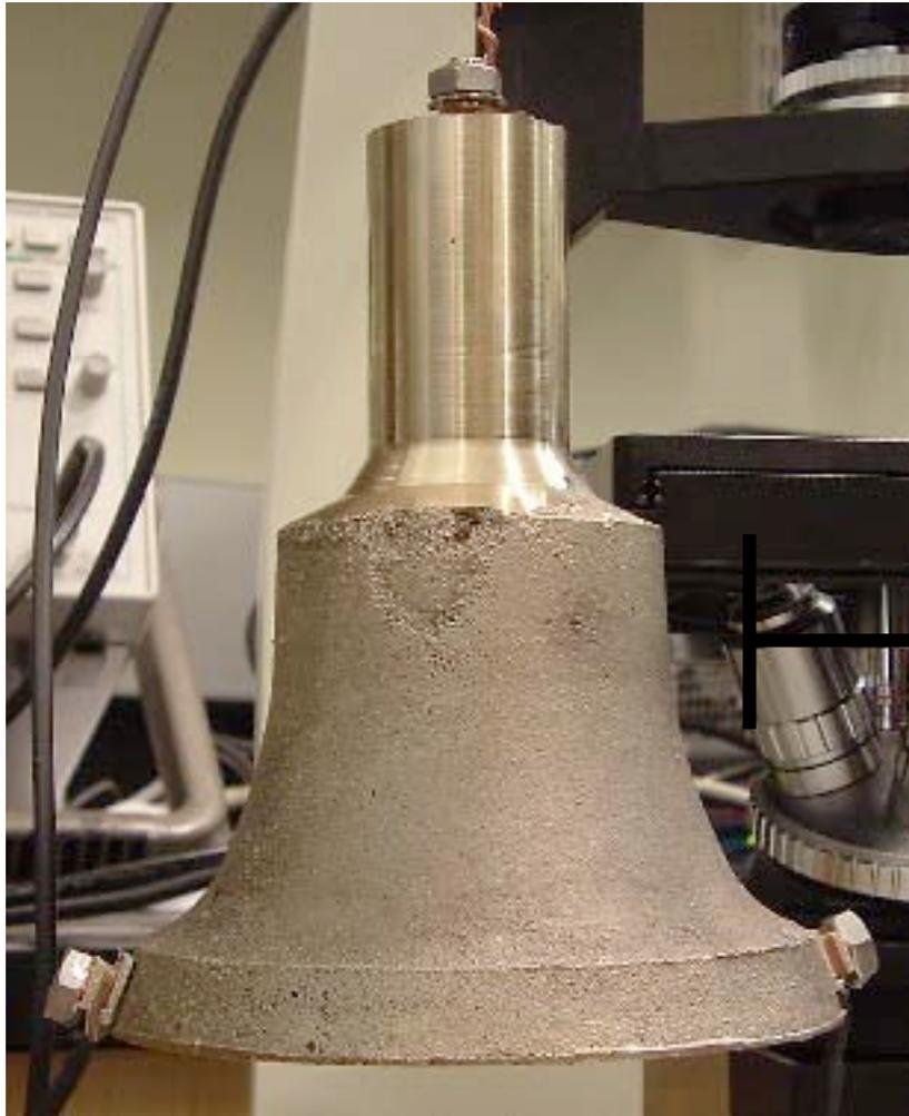
**Localized heating of upper waist** - Proven in experiment that annealing provides a lower young's modulus for all three alloys. Creates a more elastic connection to (hard) crown.
