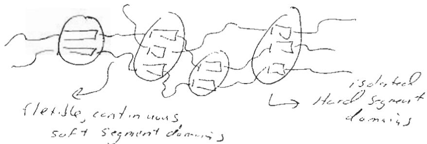
the isolated hard segments act as virtual crosslinks, thereby creating a material that is a tough elastomer (has "snap"). Any biomedical application that requires a tough flexible elastomer would be a good choice for a segmented polyurethane-area.
