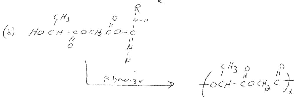
Note: activation of the acid group with carbodiimide chemistry limits the amount of ester interchange that can take place during a direct esterification reaction. Ester interchange would produce a random copolymer!
