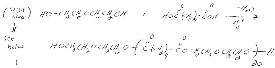
→ to synthesize a soft segment with 20 repeat units (orange), we need a polymer with 40 structural units (2 structural units per repeat unit)
