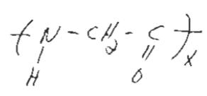
This polymer does not have any stereoisomers, nor can it be optically active; no double bonds, no  $-\overset{\text{R}}{\underset{\text{H}}{\text{C}}}-$  groups, no chiral carbon centers
