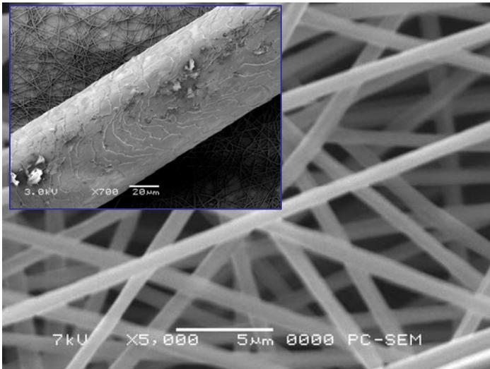
Electrospun PEO could be used for filters, composites, fuel cells, drug delivery, cell scaffolds, etc. [Rutledge Group, MIT]
