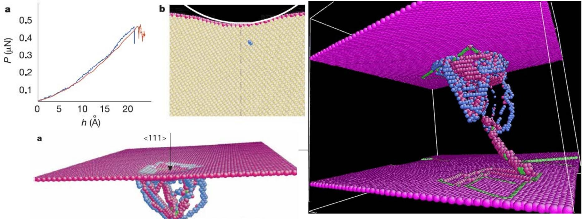
**Thin film of aluminum, moving atoms according to  $U(r)$  under distributed load of spherical indenter. Atom color = atomic coordination number.**
