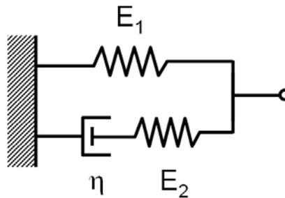
*SOLUTION: As discussed at recitation, at high strain rates dashpots act like rigid connections (springs act like springs no matter what the strain rate is). At early times and high strain rates the effective stiffness is therefore  $E_1 + E_2$ . Conversely, at long times and low strain rates dashpots act as though they aren't even connected. Under these conditions the effective stiffness is  $E_1$ .*
