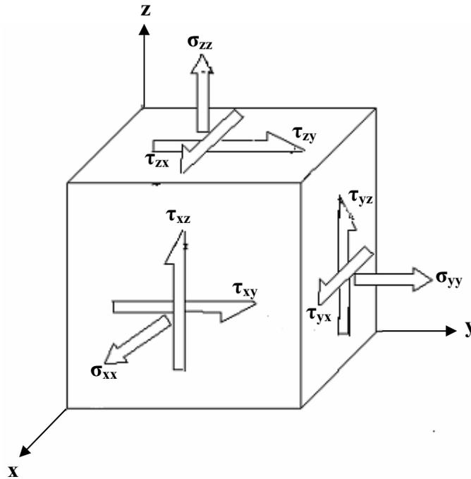
*For each of the following situations, describe the stress state in terms of a stress matrix  $\sigma_{ij}$ . Determine the principal normal and shear stresses and give the orientation of the principal axes as well as the orientation of the max shear stress.*
