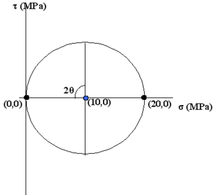
We see by simple visual inspection of the Mohr circle that we are already in the principal stress state (i.e. all shear stresses are equal to zero), so we do not need to rotate our circle (or material) any further. The principal axis is the x-axis. Also, there is only one principal normal stress which is equal to 20MPa.
