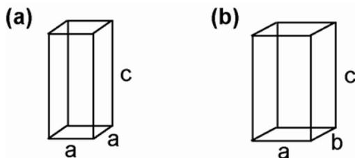
Fig. 3: Unit cells for (a) tetragonal and (b) orthorhombic crystals.
