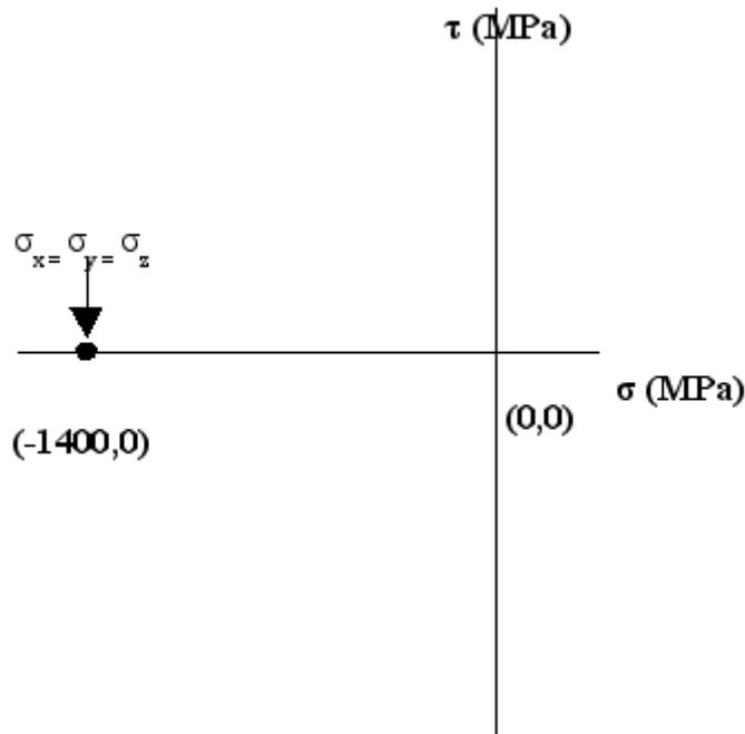
*As all of the shear forces are equal to zero, we see that we are already in the principal stress state with each of the principal normal stress being equal to -1400MPa. The principal axes are the x-, y-, and z-axes as noted in our original diagram and no rotation is necessary.*
