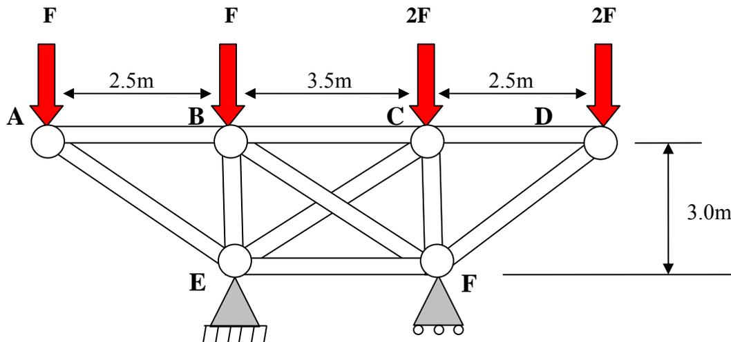
Figure 1b: Schematic of truss section with pin-loaded joints and supports.
