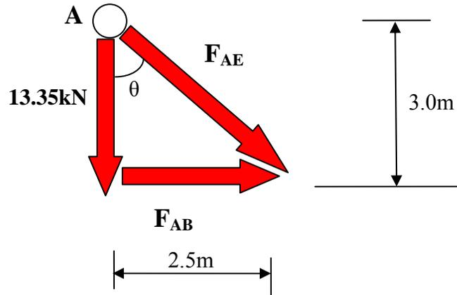
*The angle,  $\angle \theta$ , can be determined from the truss dimensions as follows*
