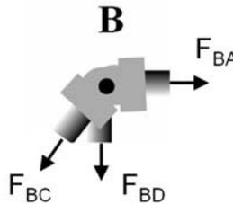
*Setting the sum of the forces in the x direction at pin B to zero:*
