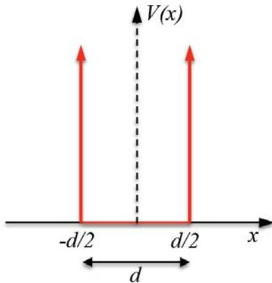
Consider the above system with the piecewise potential energy function  $V(x)$  for an electron inside the infinite potential well.
