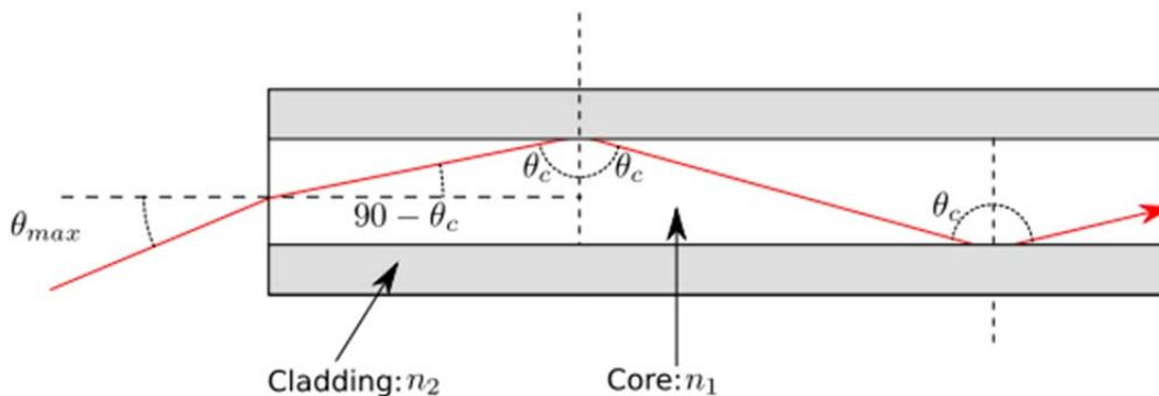
Then we can find the maximum angle at which we can still “couple” EM waves into the waveguide so we can take advantage of the total internal reflection.
