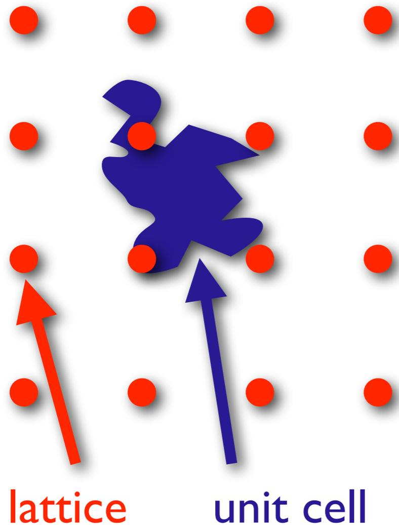
A crystal is built up of a unit cell and periodic replicas thereof.
