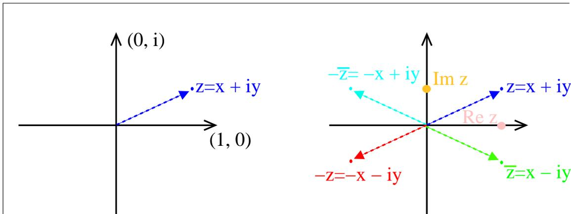
Figure 8-1: Plotting the complex number  $z$  in the complex plane: The complex conjugate ( $\bar{z}$ ) is a reflection across the real axis; the minus ( $-z$ ) operation is an inversion through the origin; therefore  $-(\bar{z}) = (-\bar{z})$  is equivalent to either a reflection across the imaginary axis or an inversion followed by a reflection across the real axis.
