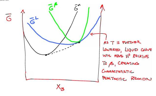
7. Shown below is a free energy vs. composition diagram for a binary system that has two different solid phases  $\alpha$  and  $\beta$ , each of which behaves as a regular solution. Use this diagram to answer the questions below:
