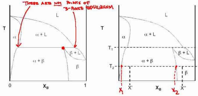
a. (3 points) On the left-hand diagram, mark the invariant point(s) and write the equilibrium that exists at each in the space below.
