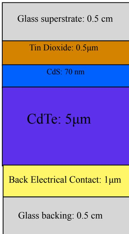
**Figure IV. 2: Schematic of our CdTe solar cell**
