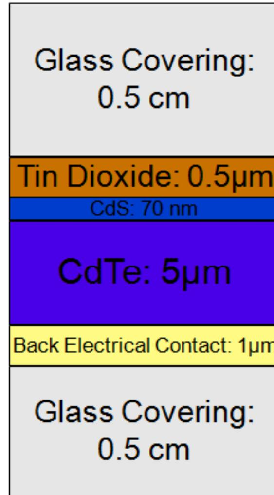
Proposed schematic for CdTe cell
