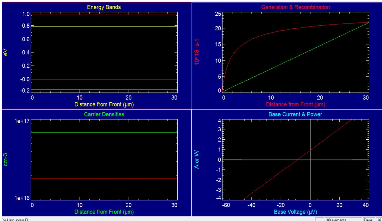
This combination yields a max base power output of  $2.09 \times 10^{-6}$  watts. We can analyze the integral of the IV curve in the fourth graph (bottom right) and compare it to the size of other combinations we try. Here we get about (10microVolts)(1Amp).
