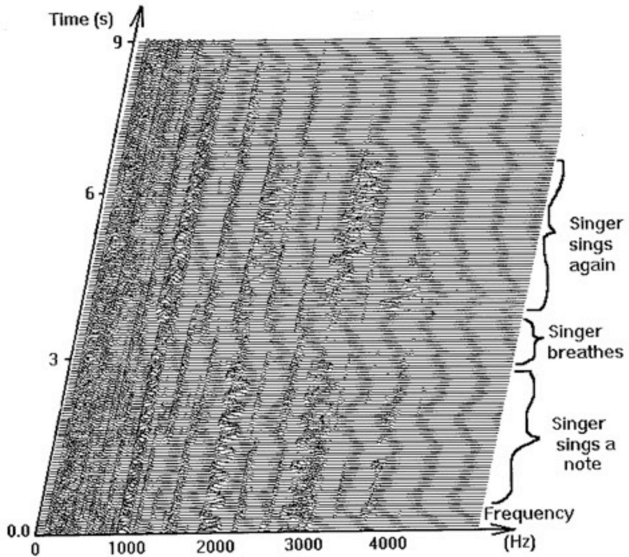
**Figure 11.12** The singer's formant is evident in this waterfall plot of the last two notes of the soprano aria "Un Bel Di Vedremo," from Puccini's *Madame Butterfly*. Common frequency modulation of the first three partials allows the fundamental to be picked out visually.
