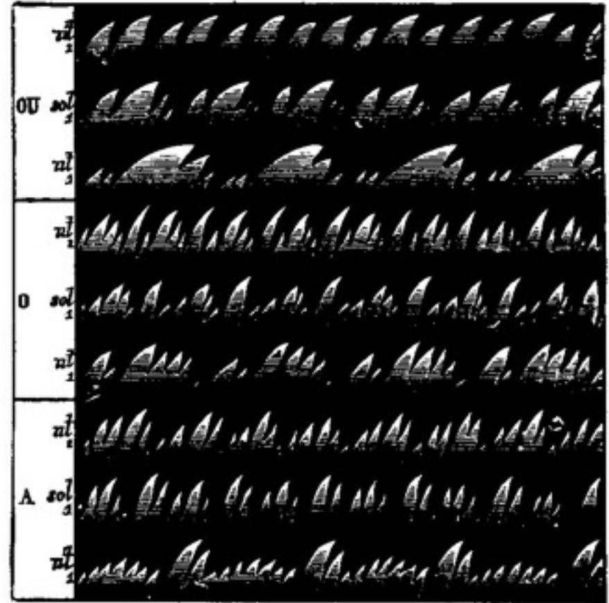
In this 19th century apparatus developed by Koenig, waveforms were visualized by viewing a flame reflected on a rotating mirrored drum. Vowel sounds resulted in the same flame pattern regardless of their pitch level.
