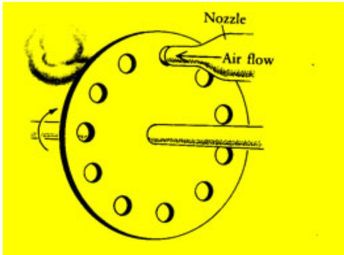
A simple siren is produced by forcing compressed air through equally spaced holes on a rotating disk. This produces a periodic vibration whose frequency equals the rate of holes passing by the air nozzle.
