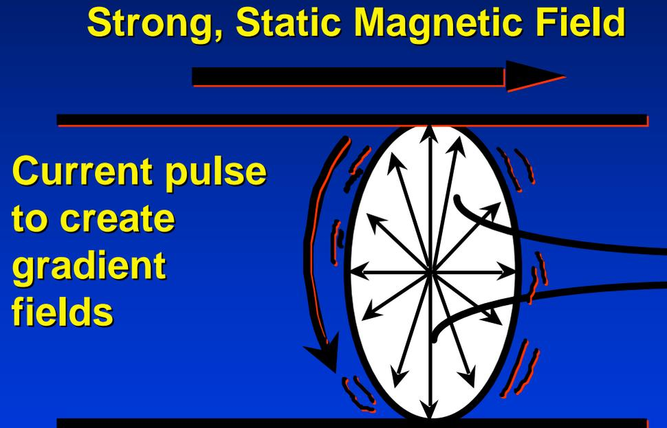
Together, these produce mechanical forces on the coils that create the gradient fields; so the coils move.
