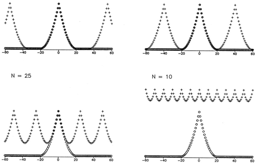
Figure 1.7: Effects of sampling at 4 different frequencies on the spectrum of a periodic signal with 39 components. Crosses show the Fourier coefficients of the sampled signal, circles those of the continuous-time signal.
