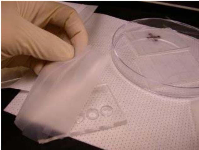
Take the PDMS device and peel off the protective tape. Now use this tape to remove any particles on the bonding surface. Pay extra care to remove particles around the fluid delivery holes as these may clog the channels if they enter the device.
