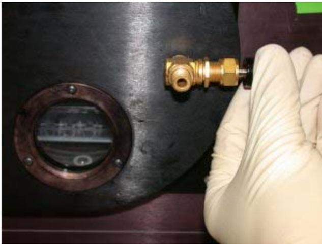
Close the door and close the venting valve on the door. Turn on the vacuum and switch on the RF generator but leave the dial for the RF strength in the off position. Wait 3 minutes to ensure a good vacuum is created in the chamber.
