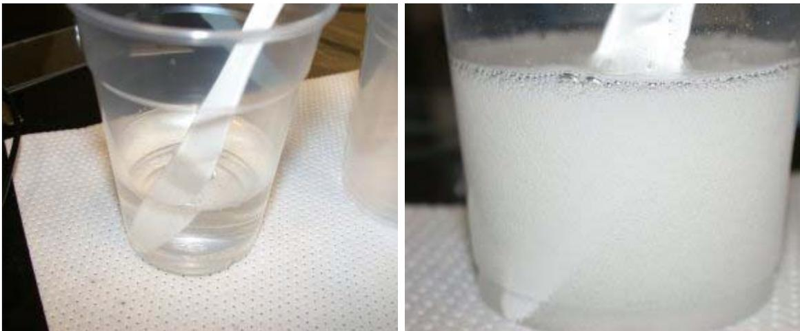
Take the cup off the scale and begin to stir the PDMS mixture using the disposable plastic knife. Stir the mixture for approximately 3 minutes. A large stopwatch is useful for keeping time. In general, any stiff disposable rod can be used to stir the mixture and a plastic knife is low cost and works well. After the 3 minutes of stirring the mixture will have many air bubbles. These bubbles must be removed before the PDMS can be used to make a device. Throw away the knife, it is no longer needed.
