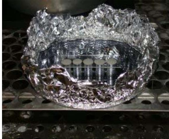
Other researchers may be baking PDMS so remember to write your name and the time you placed the PDMS into the oven on the board nearby. The curing process takes a minimum of 4 hours but optimally the PDMS should be left in the oven overnight for 8 hours.
