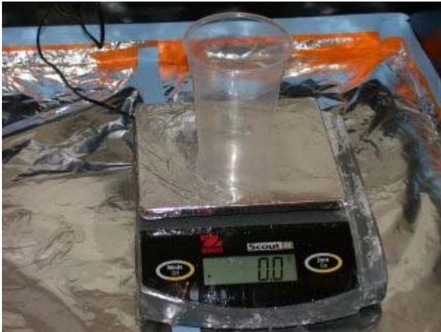
Turn on the electronic scale and adjust the device so that it reads the correct units, in this case we adjust it to read in grams. Place the cup on the scale, and press the "Tare" button to rezero the scale.
