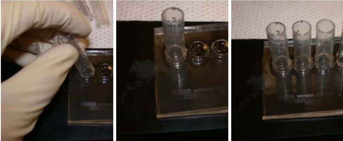
For the reservoir type devices, precut syringe tubes are inserted into the reservoir holes. When you insert the syringe tubes, be very careful not to crack the PDMS around the reservoir holes. These cracks can easily propagate through the PDMS and cause a leak.
