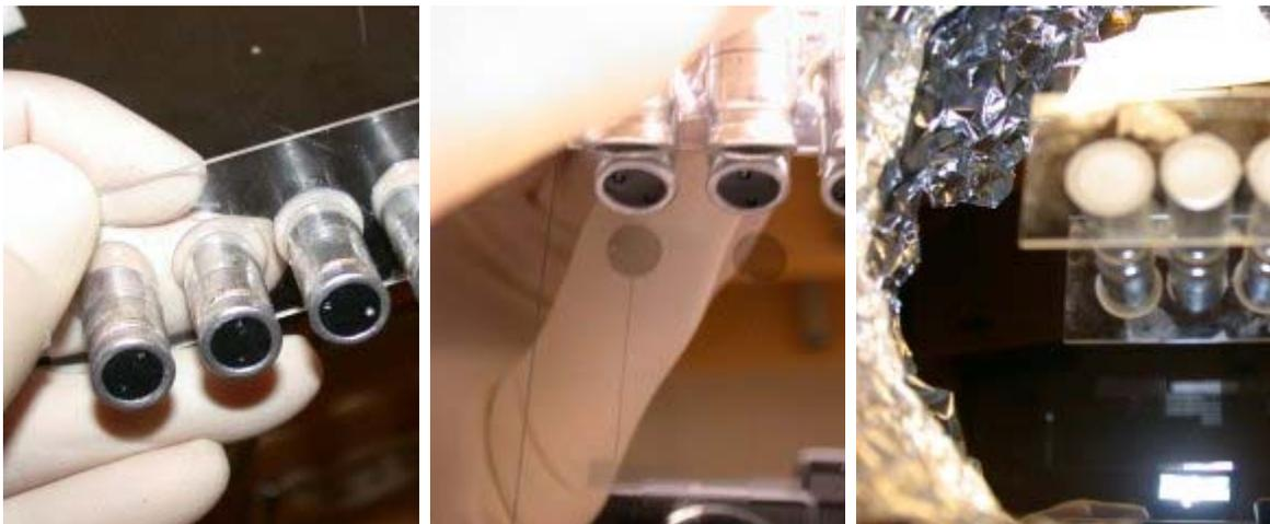
If the device requires O-Ring reservoir fittings, the O-Ring mold must be placed on the wafer before pouring the PDMS onto the master. The O-Ring mold consists of an array of capacitors glued onto a glass slide. Holding the mold with the glass slide on top and the capacitors on bottom, gently align the capacitors with the array of reservoir pads on the wafer.
