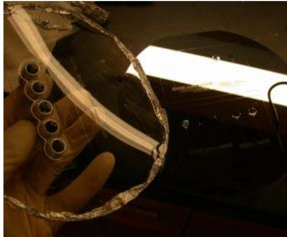
If the device uses O-Ring molds, these must be gently pried off the surface of the wafer along with the surrounding PDMS. You can pry the O-Ring mold off by tilting the glass slide gently causing the capacitors to separate from the wafer. Do this slowly as this process can place a lot of stress on the wafer. Place the peeled off PDMS on the lab bench with the side containing the channels face up.
