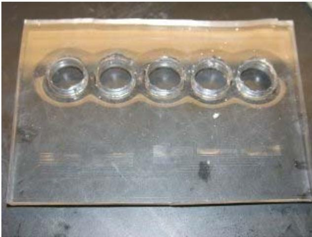
After the O-Ring mold has been removed or if the device uses pipettes or non-O-Ring reservoirs, take a box cutter and cut out the devices from the PDMS. If we are making O-Ring devices no additional post processing is required.
