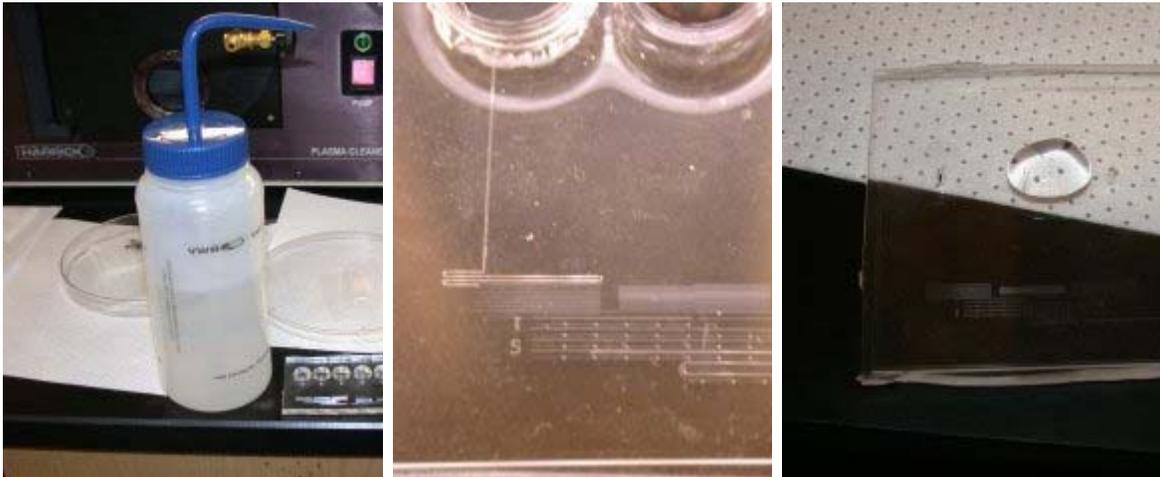
The device should be filled immediately with distilled water after the bonding process. After bonding, the channels are still very hydrophilic and makes it very easy to fill. Place a bead of water in one of the reservoir or punched pipette holes. You should be able to see the water from the single delivery channel fill the entire device.
