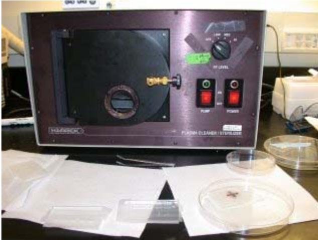
The cleaned glass slide will be bonded to the PDMS device using a plasma bonder. Inside the plasma bonder, the bonding surfaces of the slide and the PDMS device are subjected to high energy plasma which strips away electrons on the surface. This causes the surfaces to become hydrophilic. When these two hydrophilic surfaces come into contact they form a strong bond. In this project a plasma is created from air but a stronger bond may be created if a pure oxygen plasma is used instead.
