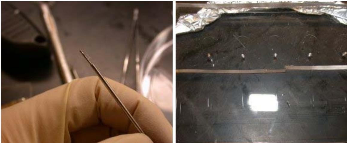
Push the needle completely through the device and use the thin rod to punch out the PDMS inside the needle before removing the the needle. For non O-Ring reservoir devices, place PDMS on a Teflon block and use a number 6 cork borer to punch a hold where the reservoir pads are located. Again try to punch the hole perpendicular to the device.
