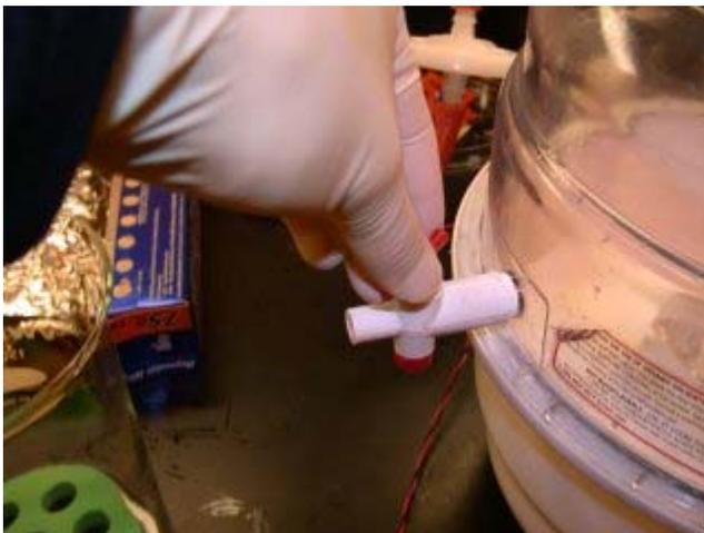
Close the lid of the dessicator and adjust the vaccuum valve on the dessicator to connect the vaccuum line.
