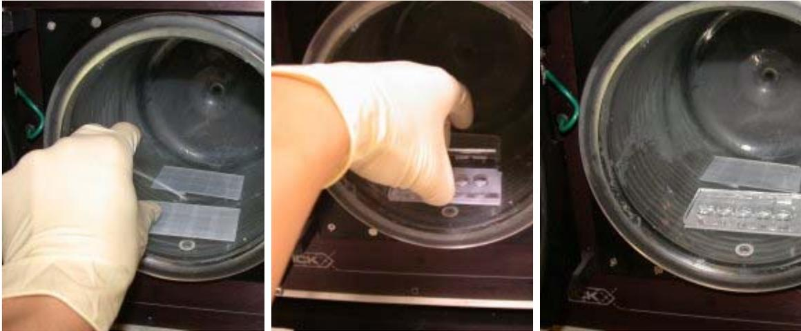
Once the surface is clean place the PDMS on a glass slide with the bonding surface face up and place the slide and PDMS into the plasma bonder. Take the cleaned glass slide and place it on another glass slide, again with the bonding surface face up and put both into the plasma bonder.
