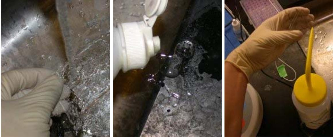
First the slides are rinsed under running water. Then clean the surface using dish detergent and rinse the soap off completely. Next rinse the surface with distilled water. Finally rinse the surface with isopropyl alcohol.
