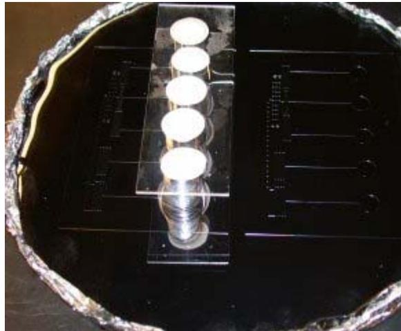
Remember to be very gentle with the wafer throughout the unmolding process. Most master breakages occur during this step. While wearing gloves, take the wafer out of the oven and place it on the lab bench. Wait a few minutes for the wafer to cool. To it easier to handle the wafer, remove the excess aluminum foil around the edges of the wafer.
