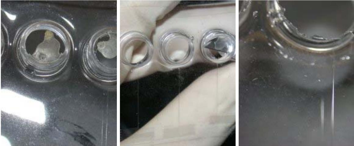
After the O-Ring mold is removed, there may still be a thin film of PDMS left over. This thin film will prevent the reservoir from feeding the delivery channel. Using a small knife, i.e. exactoknife, remove the film to bring the large reservoir in contact with the tiny delivery channel.
