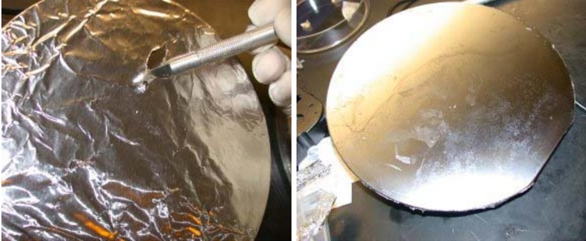
Now use a small knife, i.e. an exactoknife, to completely remove the foil on the bottom of the wafer.
