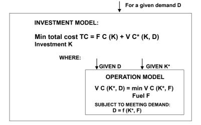
D: demand; K: installed capacity; F: fuel supply K\*(Q): optimal investment; VC\*(K,Q): optimal operation
