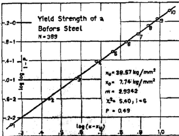
FIG. 1 YIELD STRENGTH OF A BOFORS STEEL
