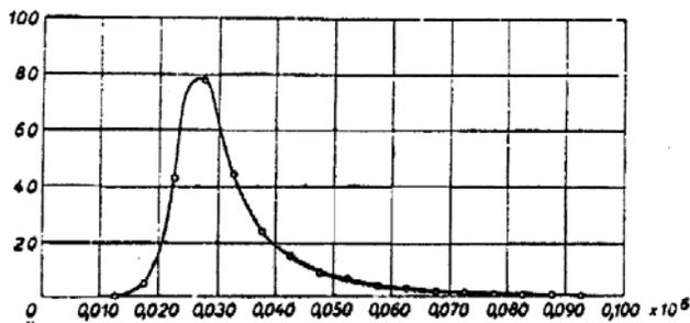
FIG. 5 FREQUENCY CURVE OF FATIGUE LIFE OF ST-37 STEEL
