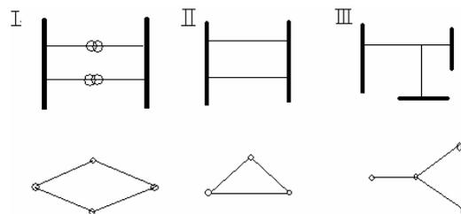
**Figure 2: Representation of elements in the network**
