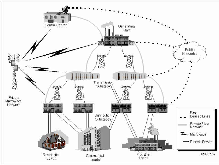
**Figure 13: Physical representation of the network**
