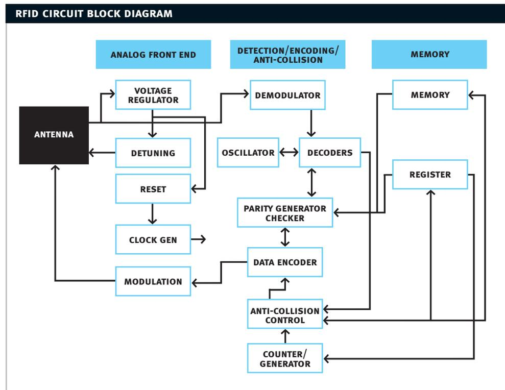
Figure 3 describes a block diagram for RFID IC circuits and lists many of its associated function blocks. The RF front end is connected to the antenna. Typically, at UHF, an electric dipole antenna is used. HF tags use a coil antenna. Passive RF tags have no power source and rely on the signal from the reader to power up. Thus the RF front-end implements modulators, voltage regulators, resets and connections to external antenna.
