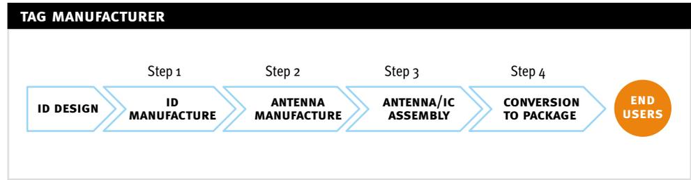
After the design of the IC, there are four steps in the manufacture of an RFID tag, as shown above.
