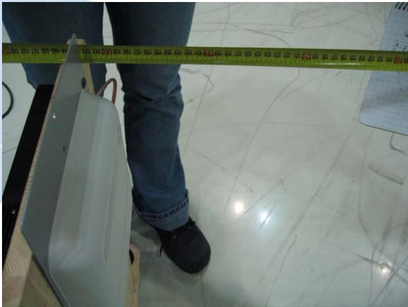
Read ranges from the surface of the reel 0.36 m – 1.4 m depending on the direction
