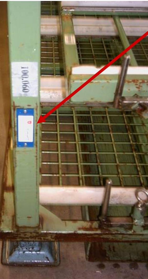
RTI's are equipped with two transponders
