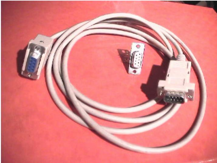
**Figure 4** Serial data connection components.
