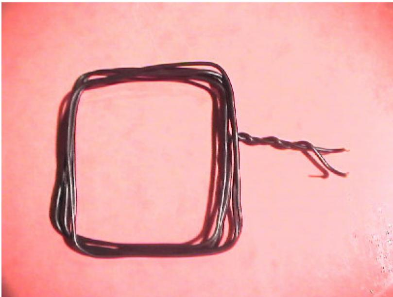
**Figure 14** Square loop antenna built with 5 square loops of regular cable. Note the twisted leads.
