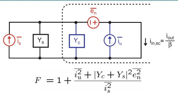
We can replace voltage and current noise currents with impedances and admittances
