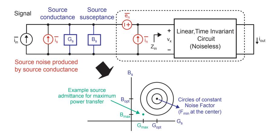
One cannot generally achieve minimum noise figure if maximum power transfer is desired
