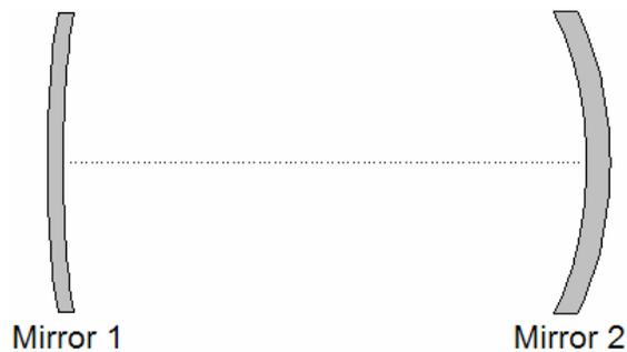
(d) (9 points) Consider the stable plano-concave resonator shown below. The fundamental mode of the resonator at wavelength  $\lambda = 1\mu\text{m}$  is a Gaussian beam with the waist radius  $w_0$ .
