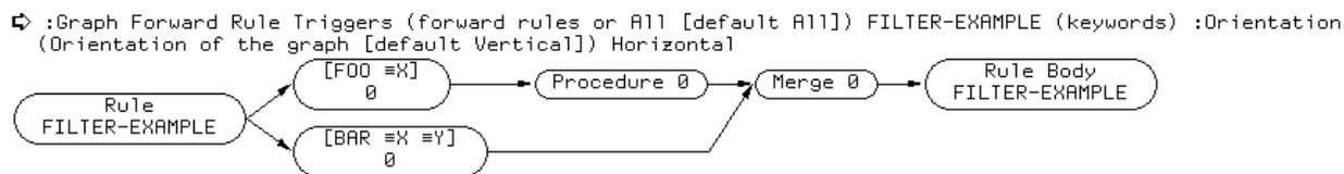
Figure 13. Sample Rete Network Display with Filter Nodes
