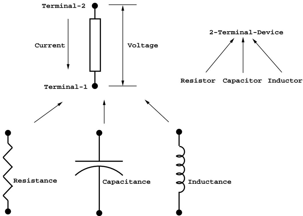
Figure 38. The Object-Type Hierarchy of Two-Terminal Devices
