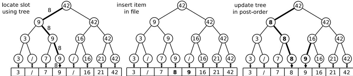
Figure 2: Inserting the key '8' in the data structure.
