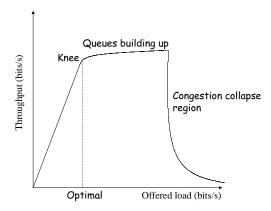
Figure 2: Schematic view of throughput vs. offered load, showing the optimal operating point and congestion collapse region.
