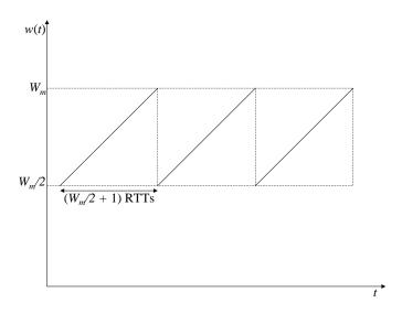
Figure 4: The steady-state behavior of the TCP AIMD congestion window.
