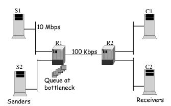
Figure 1: A simple network topology showing how sharing causes resource contention. Many connections between senders and receivers contend for the bottleneck 100 Kbps link.
