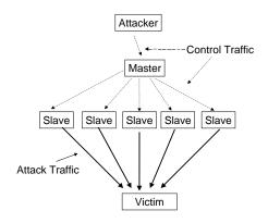
Figure 1: Architecture of bandwidth attacks.
