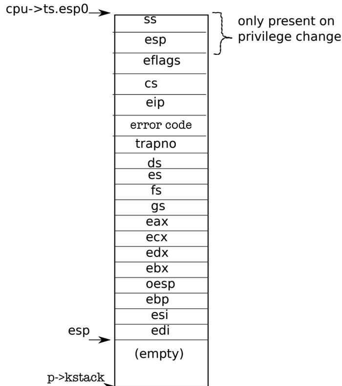
Figure 3-2. The trapframe on the kernel stack
