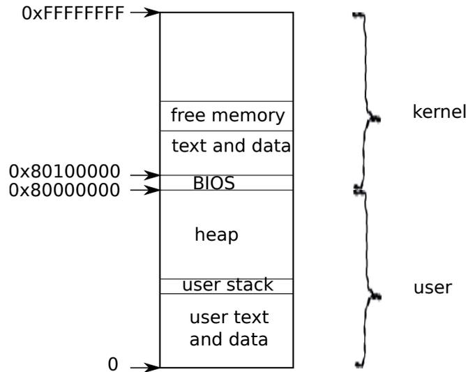
Figure 1-1. Layout of a virtual address space
