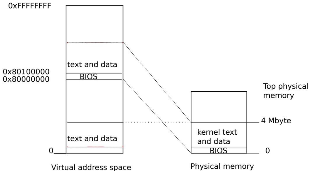
**Figure 1-2.** Layout of a virtual address space
