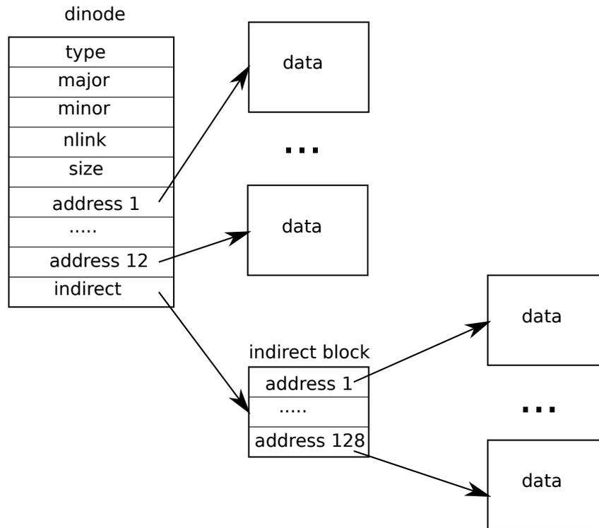
**Figure 6-4.** The representation of a file on disk.
