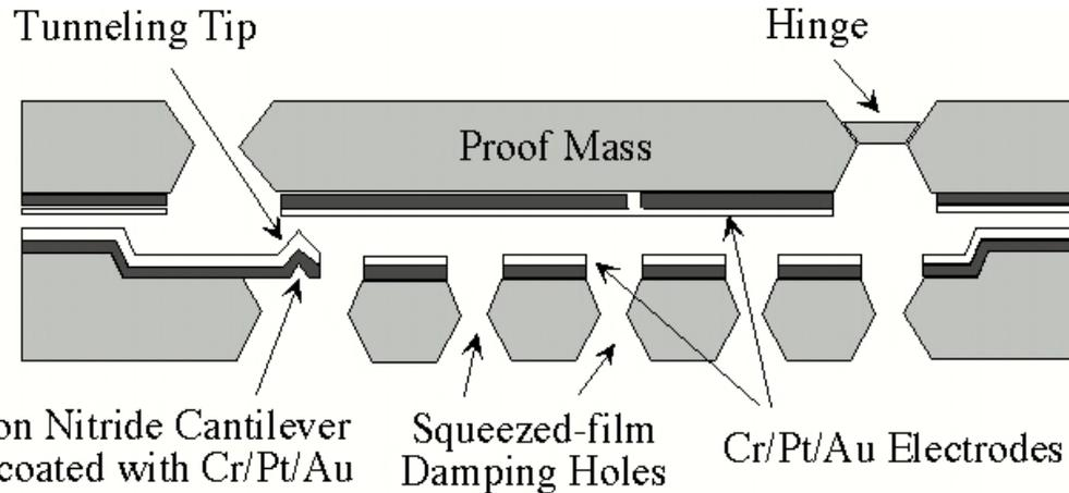
Nitride cantilever with tunneling tip
