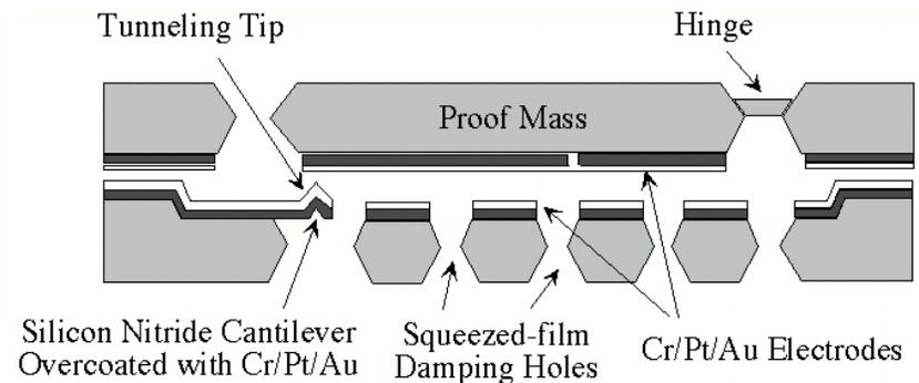
Figure 2 on p. 236 in Liu, C.-H., A. M. Barzilai, J. K. Reynolds, A. Partridge, T. W. Kenny, J. D. Grade, and H. K. Rockstad. "Characterization of a High-sensitivity Micromachined Tunneling Accelerometer with Micro-g Resolution." *Journal of Microelectromechanical Systems* 7, no. 2 (June 1998): 235-244.
