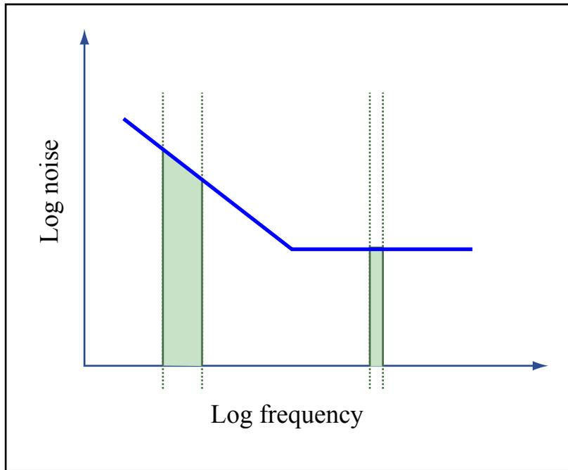
**Same noise bandwidth, but lower spectral density at the higher carrier frequency**
