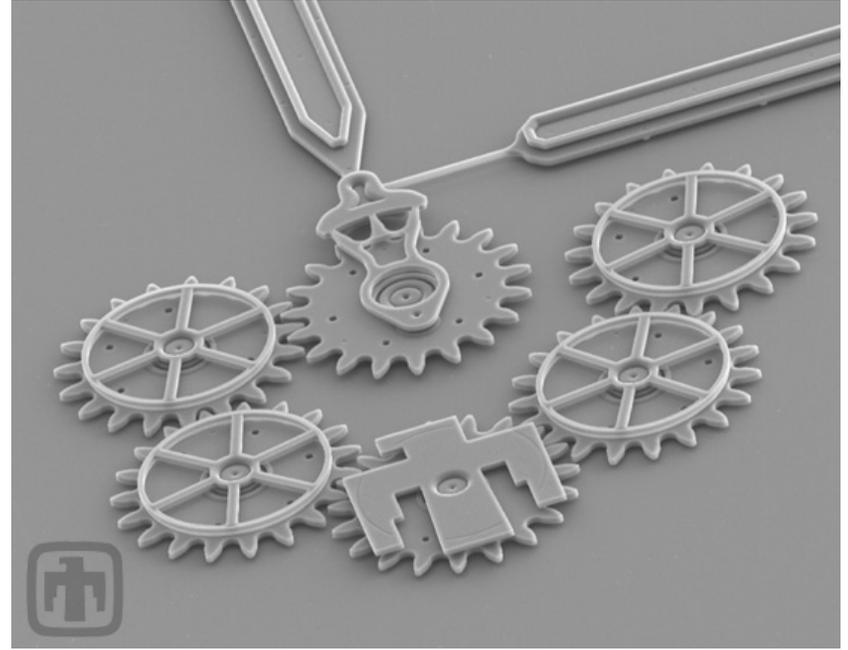
**In-plane processing; potentially out of plane structures.**
