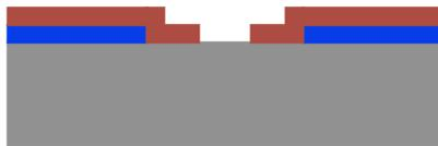
4. Strip resist; pattern with new resist mask
