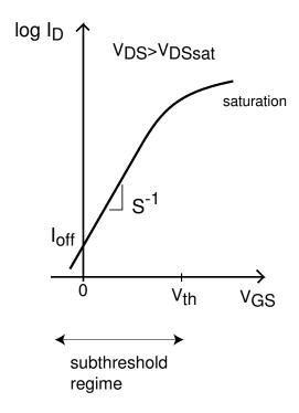
From these experimental characteristics, one can extract important parameters of a MOS-FET. For this exercise, use the long-channel description of the I-V characteristics of a MOSFET:
