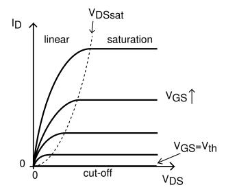
The slope of the drain current with  $V_{DS}$  is the *output conductance*  $g_d$ , which graphed as a function of  $V_{DS}$  looks like:
