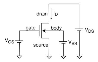
The output characteristics of the MOSFET refer to a graph that shows the drain current,  $I_D$ , vs. the drain-source voltage,  $V_{DS}$ , with the gate-source voltage  $V_{GS}$  as parameter:
